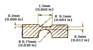
LIVING HINGE DESIGN FOR POLYPROPYLENE AN POLYETHYLENE
