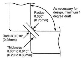
**Figure 3:** Dimensions for a right angle hinge.
